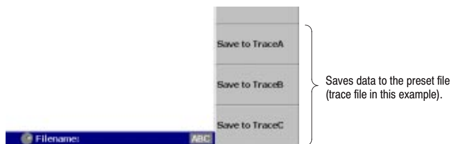
Figure 3–105: Save to the preset file (lower right of the screen)
