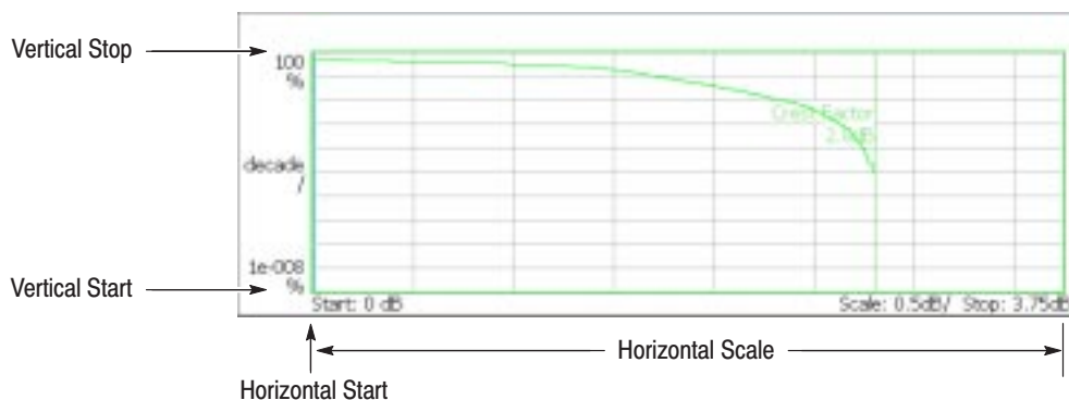
Figure 3–49: Setting the scale in CCDF view
